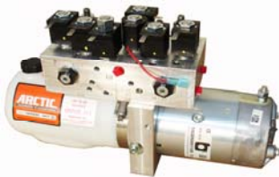
Power unit 2012+ - Pump used FP12171-380-SA - a relief valve setting at 1500 psi
